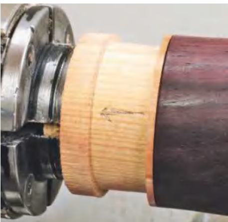
STEP 34. The base needs to be reversed onto a jam chuck so you can remove the spigot. To achieve accuracy and the maximum strength from the fixing, the top of the box needs to be right up against the shoulder
